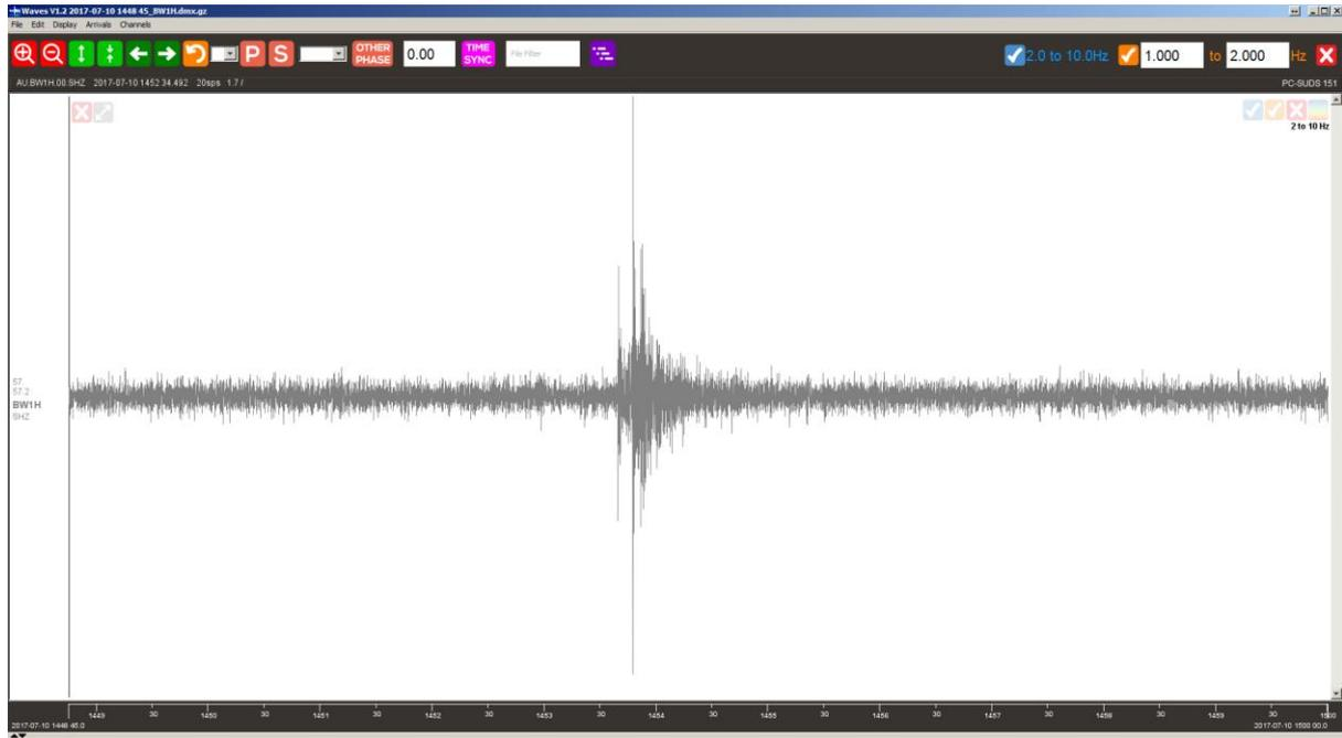
Figure 23: Example of an ML 1.8 aftershock
