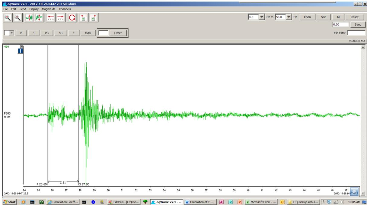
Figure 16: Earthquake recorded on FS03 on 26 October 2012.
