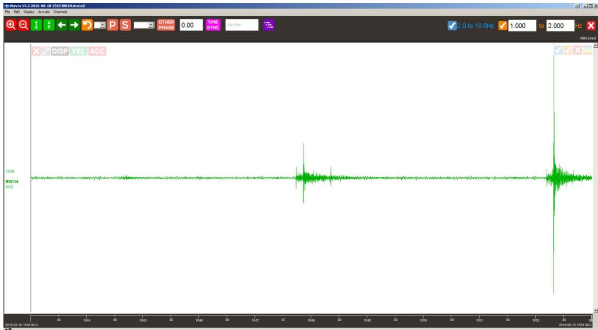
Figure 24: Example of ML 2.2 and ML 2.6 aftershocks.
